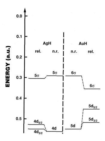
Figure 1. Orbital energies of the diatomic molecules AgH(g) and AuH(g) from relativistic and nonrelativistic calculations. Energies in atomic units, 1 a.u. =  $27.212\,\text{eV} = 2625.5\,\text{kJ}\,\text{mol}^{-1}$ . Thus  $\Delta E \approx 260\,\text{kJ}\,\text{per}$  step of the ordinate axis. Adapted from Pyykkö (9).
